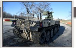
The Robotic Combat Vehicle-Light (RCV-L) experimental prototype is a small, lightweight hybrid-electric unmanned ground combat vehicle that can be transported easily by military aircraft. Its highly versatile common architecture and modular payload features offer a scalable continuum of capabilities that can be adapted to new and emerging threats well into the future
